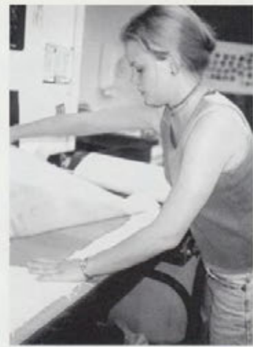
Fig. 3-30. When the clay is flattened, she reverses the direction of the wheel and rolls it back over the clay until the roller clears the slab, then removes the top canvas. The bottom canvas functions as a sling for carrying the slab to a work table.
