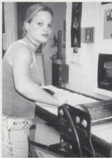
Fig. 3-29. Barbara Fransway uses a mechanical slab roller to quickly roll out a clay slab. She presses wedged clay evenly by hand to about 1" and places it on the roller atop a piece of canvas. Then she covers the clay with a second piece of canvas and turns the wheel.
