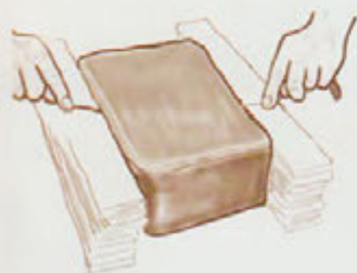
Slicing slabs with wire.
